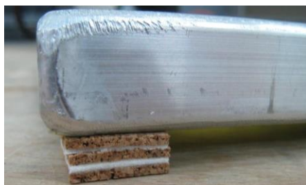
Figure 4 : Example of off-contact made with cork pad.
